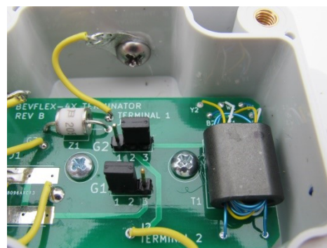
Figure 4. EWE/Flag Jumper Configuration
